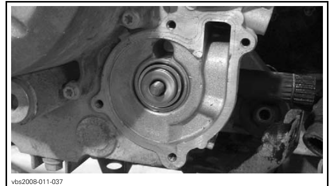
ROTARY SEAL PROPERLY SEATED ON CRANKCASE
