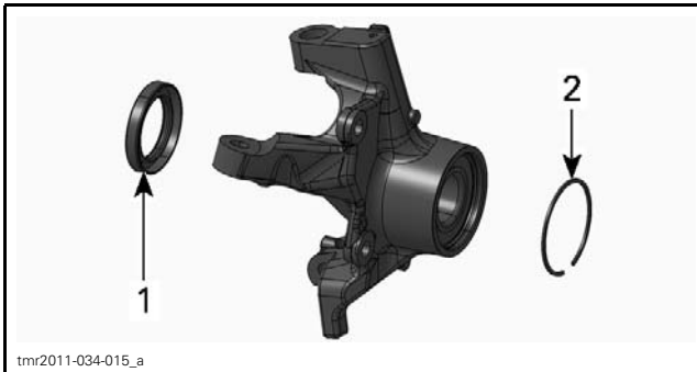
TYPICAL 1. Seal 2. Circlip
