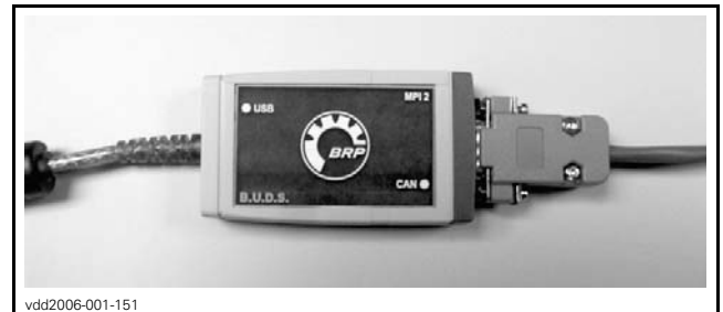
DIAGNOSTIC CABLE CONNECTED TO MPI-2 INTERFACE CARD
