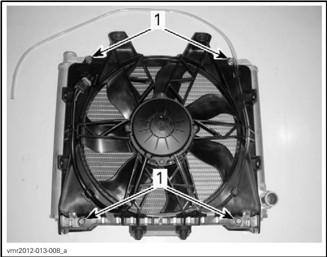
1. Cooling fan retaining screws
