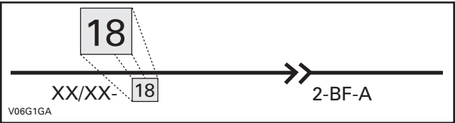
THE SHADED PART INDICATES THE WIRE GAUGE
