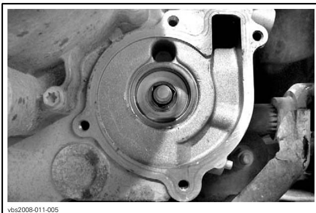
TYPICAL - INNER PART OF ROTARY SEAL REMOVED
