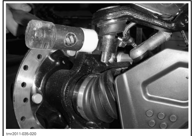
TYPICAL - CAREFULLY HIT ON KNUCKLE SIDE
