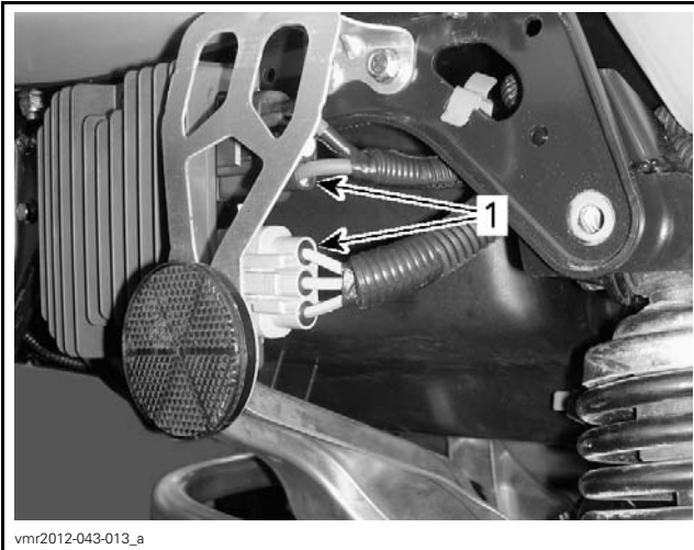
1. Voltage regulator rectifier connectors
