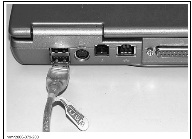
MPI-2 INTERFACE CARD CONNECTED TO USB PORT
