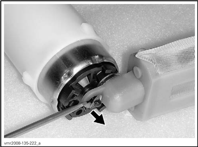
TYPICAL - FUEL PUMP 1. Fuel level sender
