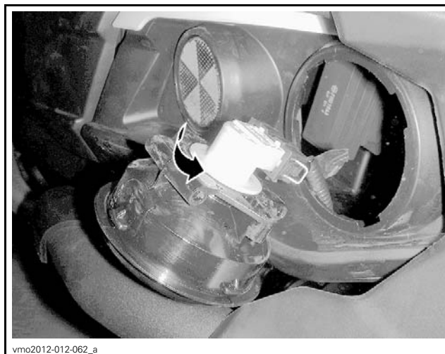
ROTATE BULB COUNTERCLOCKWISE
