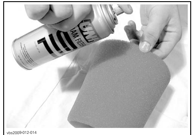
TYPICAL - OIL THE FOAM FILTER
