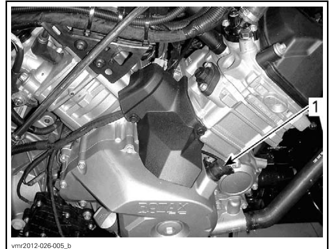
RH SIDE OF VEHICLE 1. CPS
