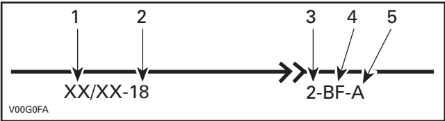
1. Wire colors 2. Wire gauge 3. Connector housing area 4. Connector identification 5. Wire location in connector
