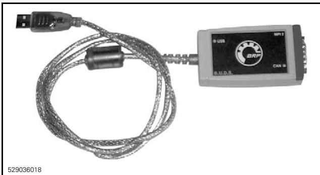
MPI-2 INTERFACE CARD CONNECTED TO USB PORT
