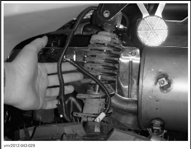
TYPICAL - LH SIDE TAILLIGHT HARNESS
