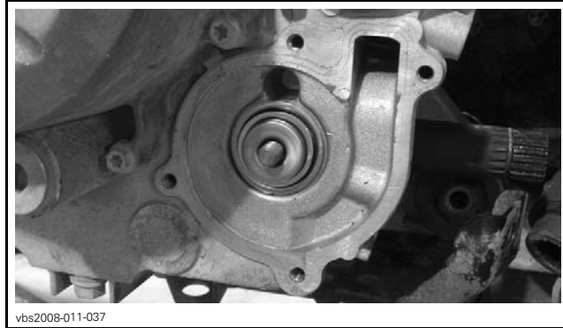
ROTARY SEAL PROPERLY SEATED ON CRANKCASE
