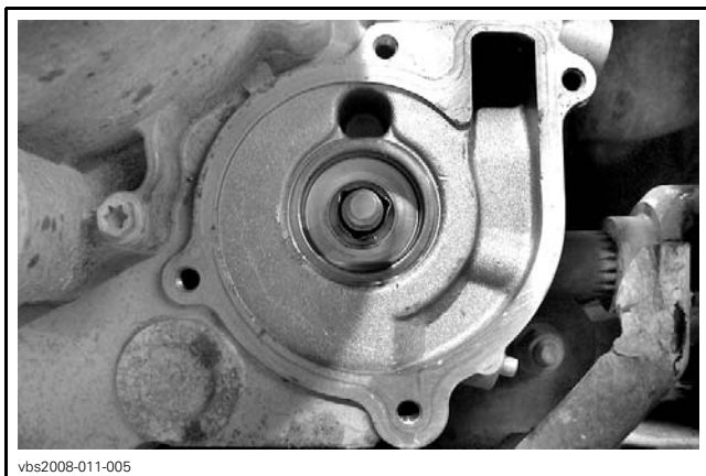
TYPICAL - INNER PART OF ROTARY SEAL REMOVED
