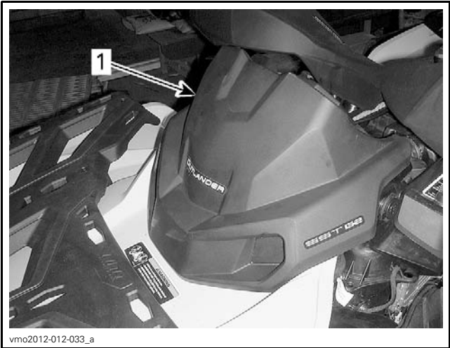
TYPICAL - OUTLANDER MODELS ILLUSTRATED 1. Gauge support
