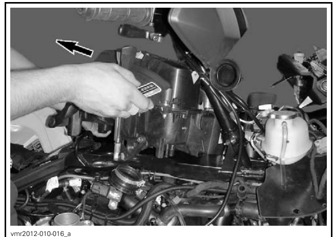
vmr2012-010-016_a AIR FILTER HOUSING REMOVAL
