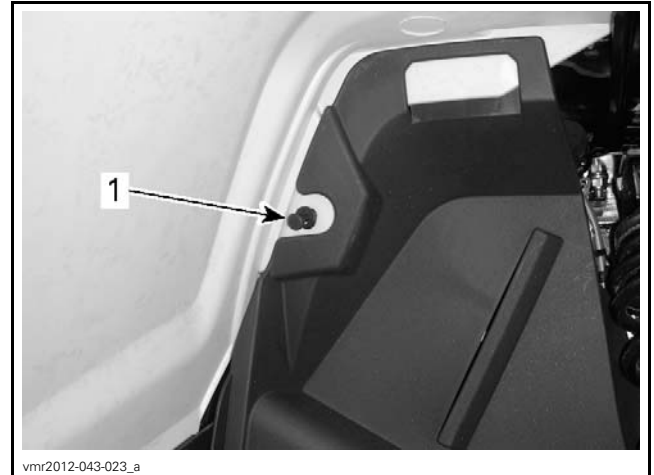
1. Plastic rivet securing side panel
