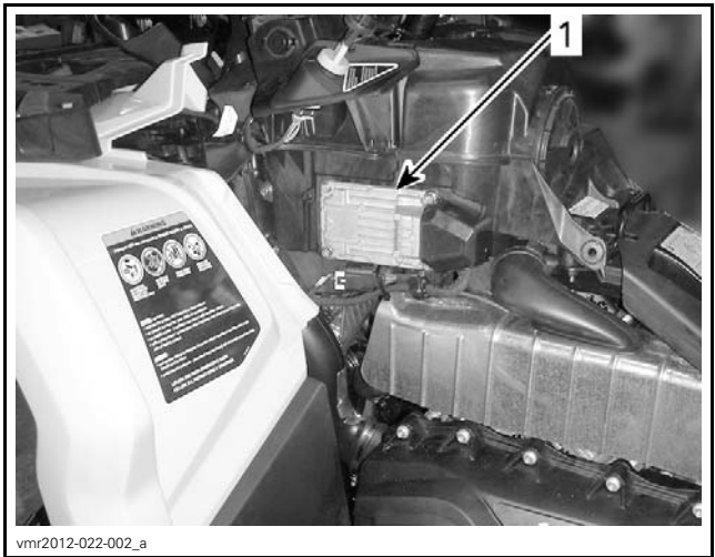
LH PANEL REMOVED 1. ECM location
