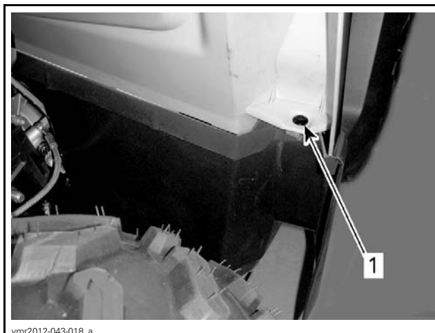
TYPICAL 1. Screw securing rear fender
