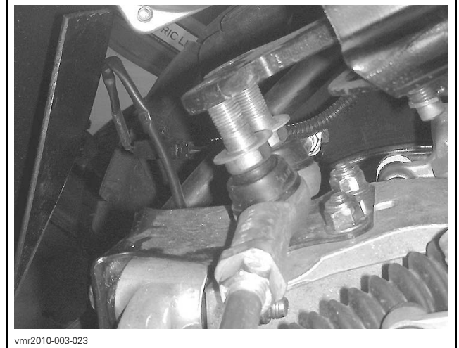
TYPICAL - TIE ROD ENDS (HARDWARE REMOVED)
