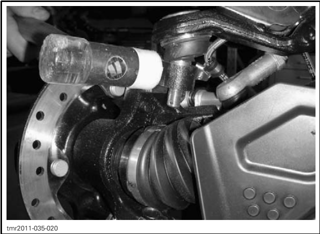
TYPICAL - CAREFULLY HIT ON KNUCKLE SIDE
