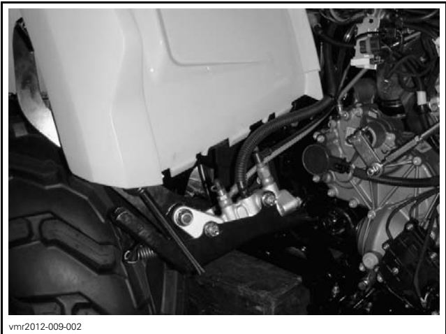
TYPICAL - MASTER CYLINDER ATTACHED ON REAR FENDER
