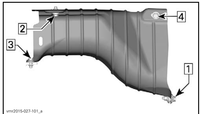
REAR HEAT SHIELD TIGHTENING SEQUENCE
