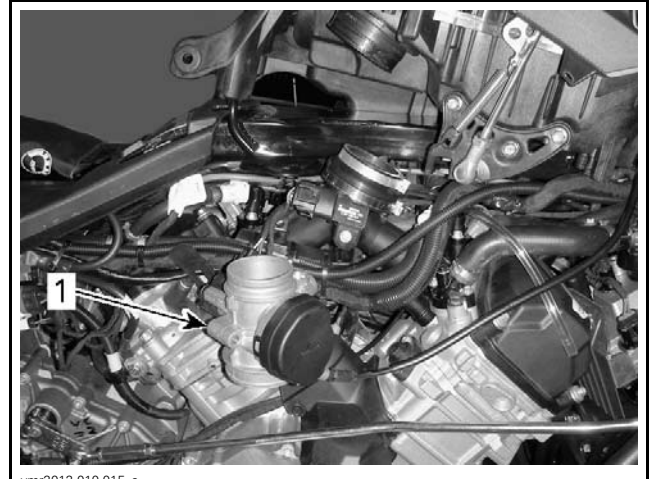
vmr2012-010-015_a TYPICAL - OUTLANDER SHOWN 1. Throttle body
