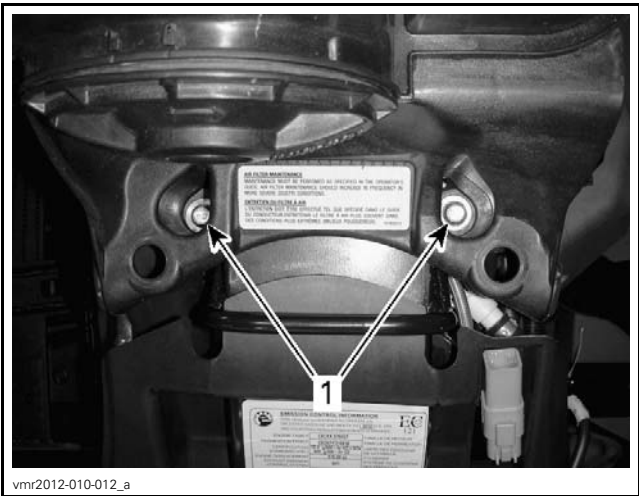
SCREWS LOCATED NEAR SEAT ANCHORAGE 1. Air filter housing retaining screws
