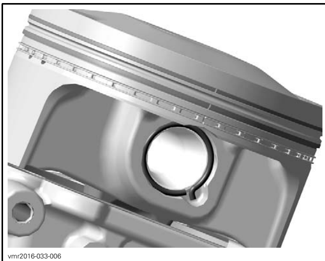
CORRECT POSITION OF THE PISTON CIRCLIP
