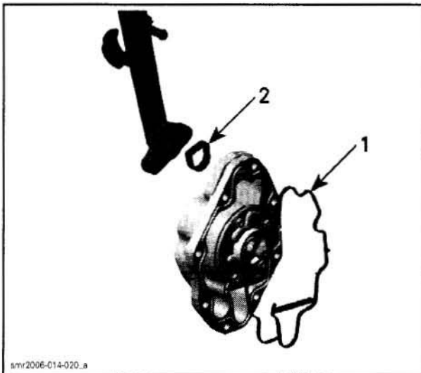
TYPICAL — NATURALLY ASPIRATED AND SUPERCHARGED ENGINES 1. Rubber ring gasket 2. Rubber ring gasket
