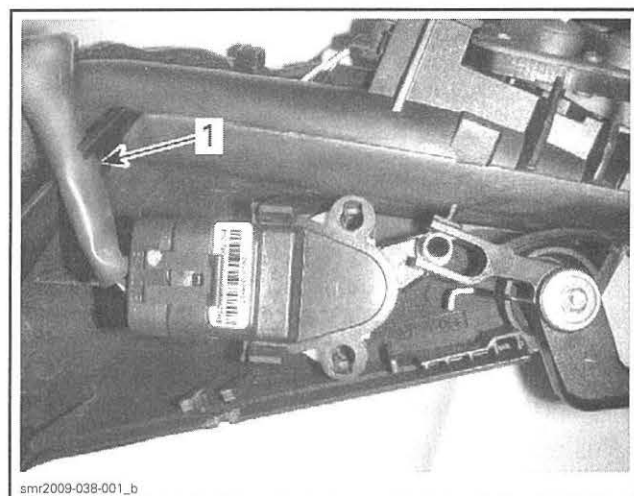
1. Wire harness routed in slot
