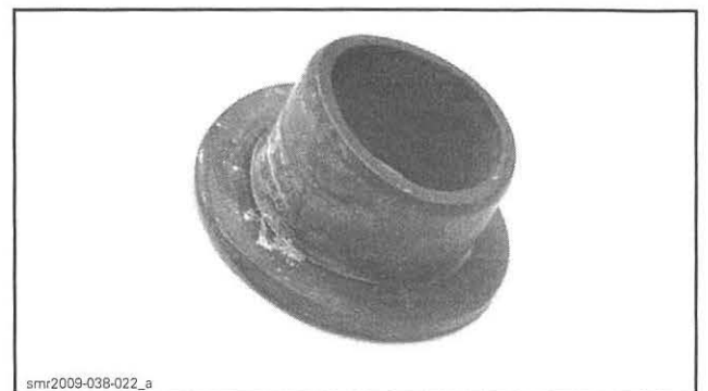
TYPICAL - WORN AND DEFORMED PLASTIC BUSHING
