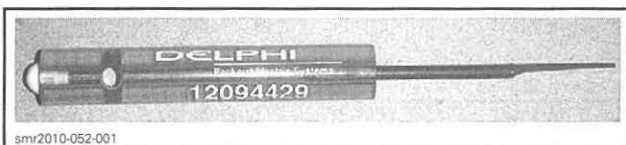
DELPHI TERMINAL EXTRACTOR (P/N 12094429)
