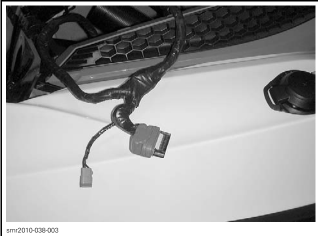
TEST CONNECTOR OF DIAGNOSTIC HARNESS
