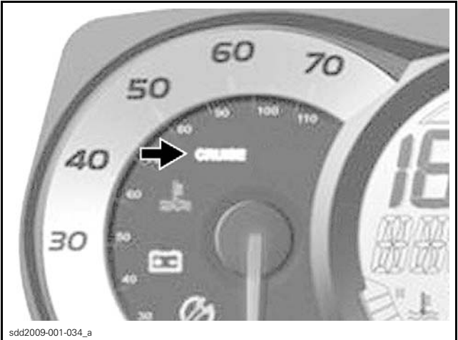
TYPICAL - CRUISE MODE INDICATOR LIGHTIN SPEEDOMETER
