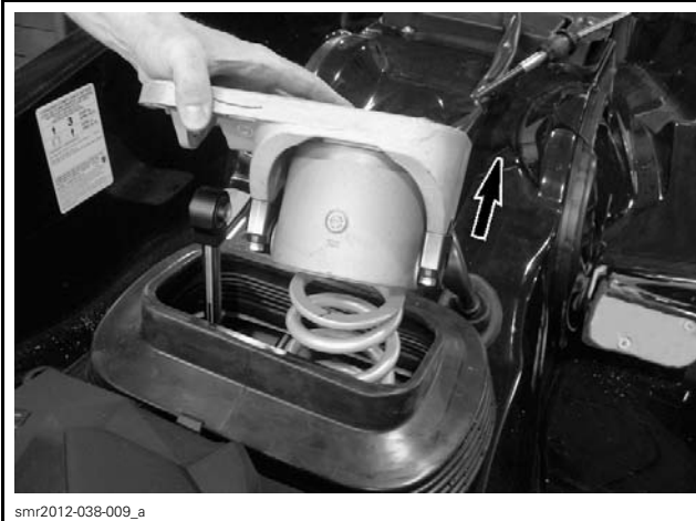
MOUNTING PLATE REMOVAL
