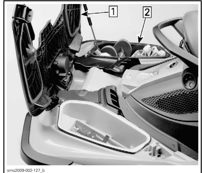
smo2009-002-127_b Step 1: Open the boarding platform Step 2: Remove the LH storage bin
