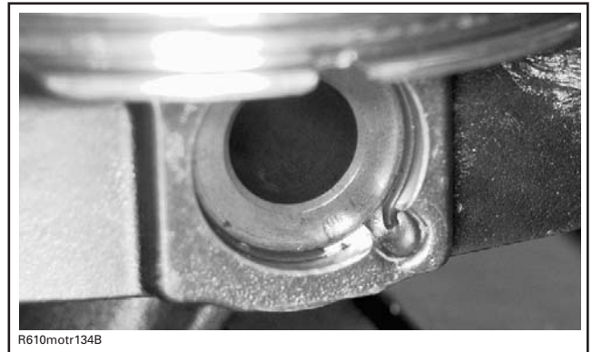
CORRECT POSITION OF THE PISTON CIRCLIP
