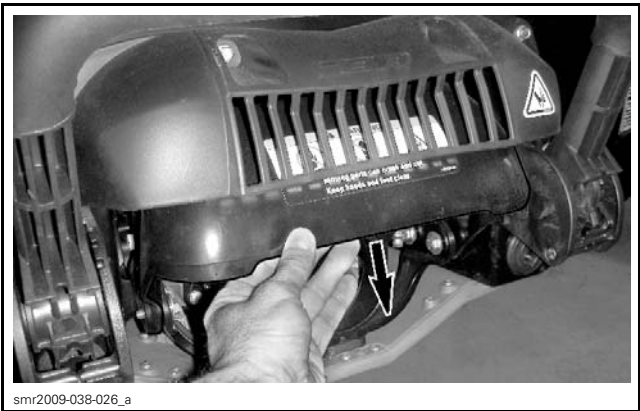
PULL DOWN SLIGHTLY ON iBR GATE
