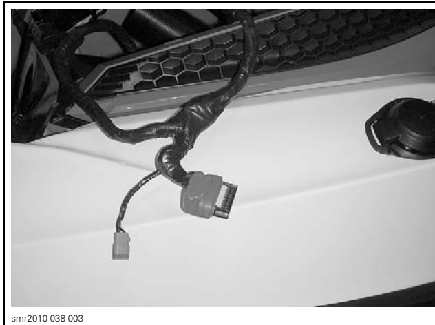
TYPICAL - TEST CONNECTOR OF DIAGNOSTIC HARNESS
