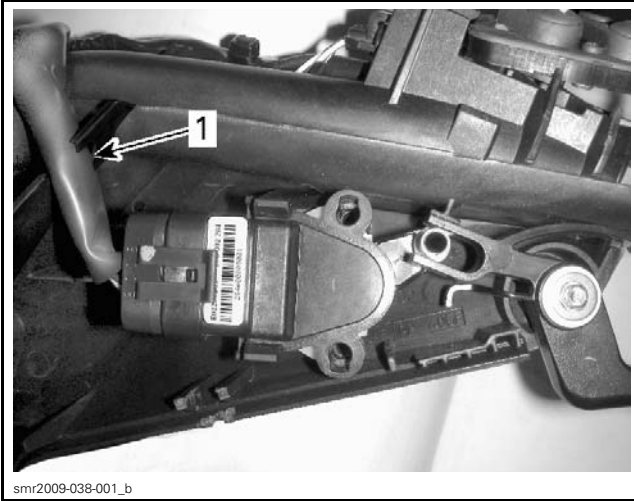
1. Wire harness routed in slot
