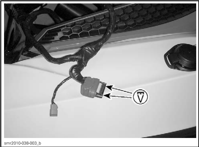
TEST CONNECTOR OF DIAGNOSTIC HARNESS
