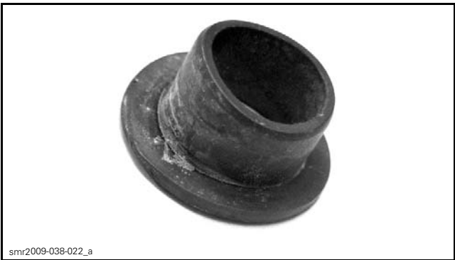
TYPICAL - WORN AND DEFORMED PLASTIC BUSHING
