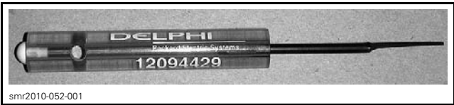
DELPHI TERMINAL EXTRACTOR TOOL (P/N 12094429)
