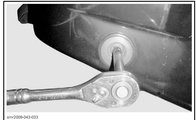
DRAIN NECK REMOVAL
