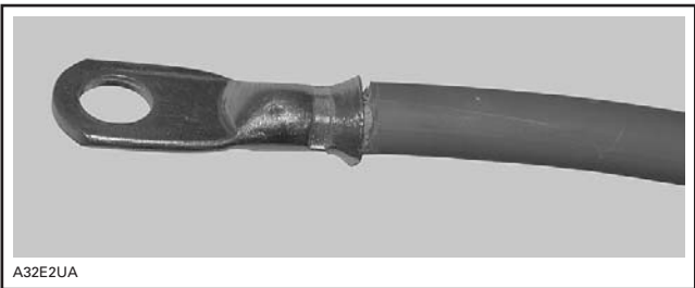
PROPERLY CRIMPED WIRE
