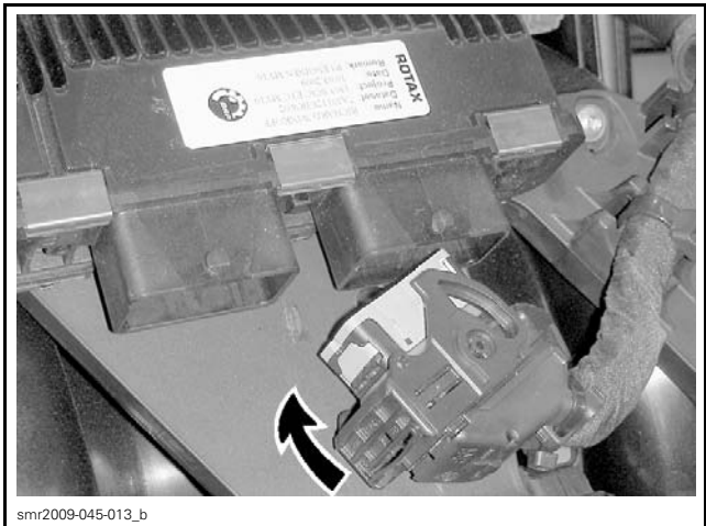
CONNECTOR LOCKING CAM IN RELEASE POSITION
