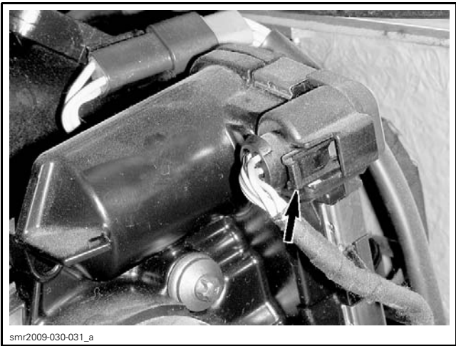
TYPICAL - PRESS HERE TO UNLOCK
