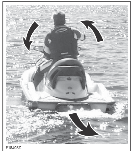
TYPICAL - STEERING DIRECTION REVERSED WHEN BACKING
