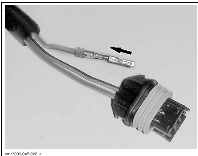
1. Red secondary lock (shown out) 2. Latch lever
