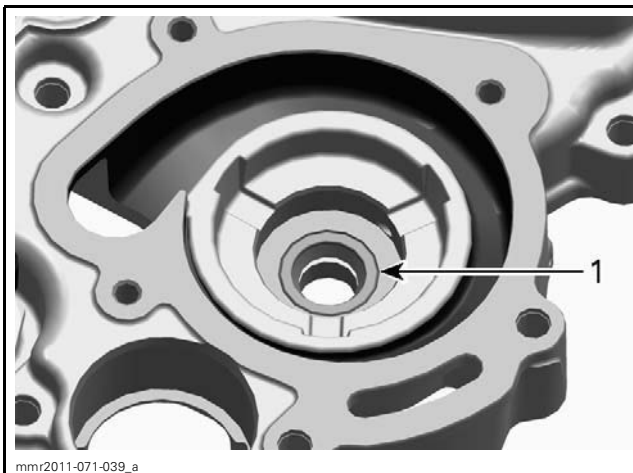
1. Oil seal correctly installed
