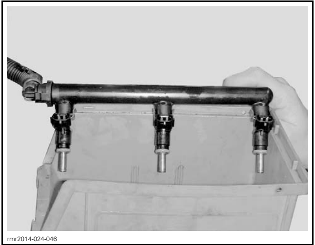
TYPICAL - INJECTOR LEAKAGE TEST SETUP
