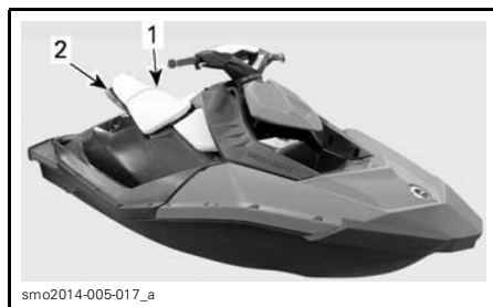
TYPICAL - PASSENGER HANDHOLDS
