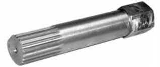
IMPELLER REMOVER/INSTALLER (P/N 529 035 820)
