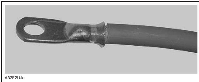
PROPERLY CRIMPED WIRE
