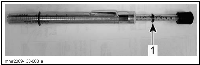
LOAD READING 1. Upper O-ring
