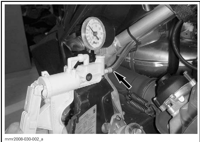
TYPICAL - VACUUM/PRESSURE PUMP ON VENT TUBE
