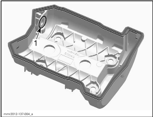
INSIDE VALVE COVER 1. Apply engine oil here
