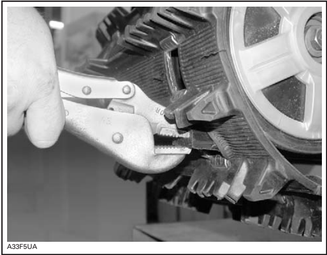
PULL ON SLIDER SHOE TO REMOVE
