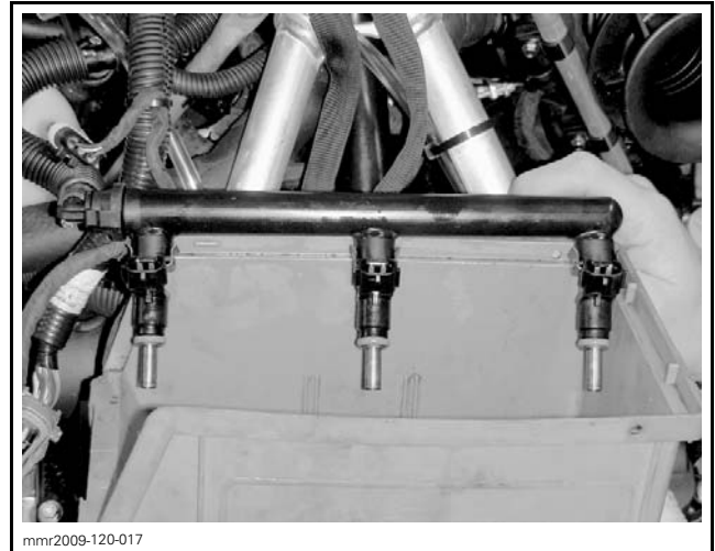
mmr2009-120-017 INJECTOR LEAKAGE TEST SETUP
