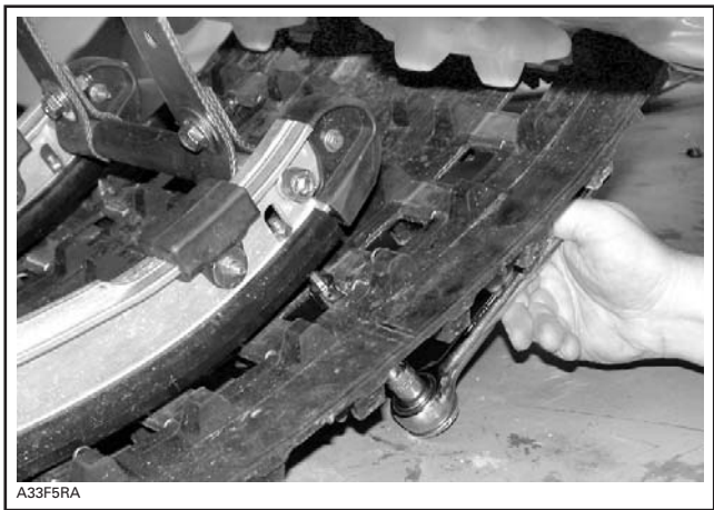
REMOVE NUT AND SCREW OF EACH RUNNER
