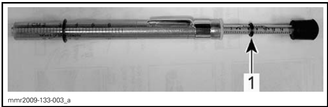
LOAD READING 1. Upper O-ring
