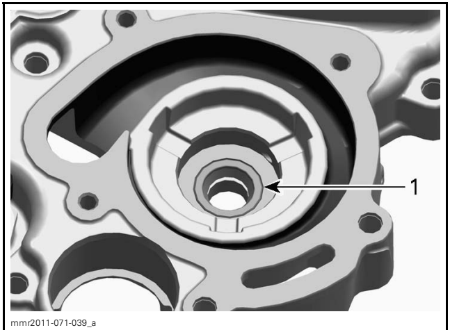
1. Oil seal correctly installed
