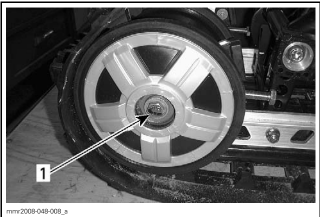
TYPICAL 1. RH rear axle screw
