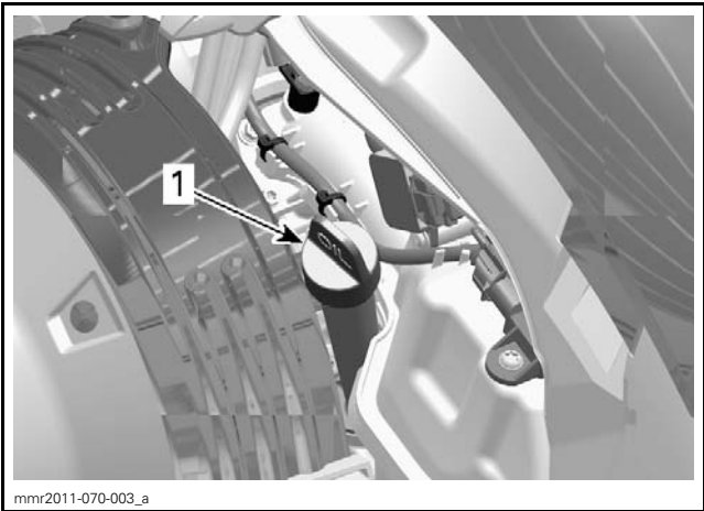
TYPICAL - LH SIDE 1. Oil tank dipstick
